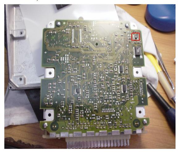
In an order type of engine control module ECM, 1 plug, one need to find the memory 24c02 marked as B58.
