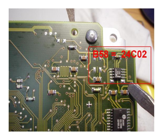
In memory 24c02 in address 38 and 39 type 2A 4E and in address from 3F to 42 type 9C D4 13 56.
