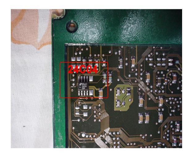
In memory 24c04 in the address 1EE to 1F9 type 2A 4E 00 00 FF FF 00 9C D4 13 56 01.
