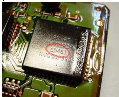
Location of mask set on the processor
