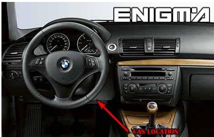
PHOTO 1: Locate the CAS2 module in the car.
