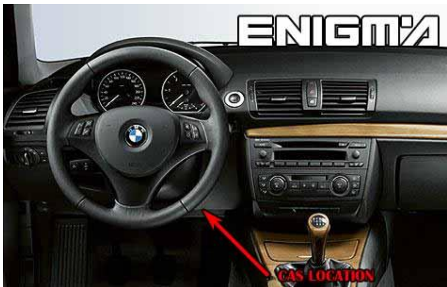
PHOTO 1: Locate the CAS2 module in the car.
