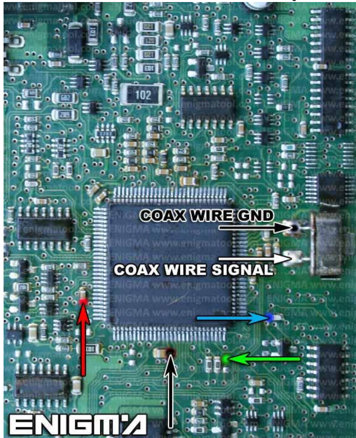
PHOTO 3: Solder C45 cables as shown on the photo above.
