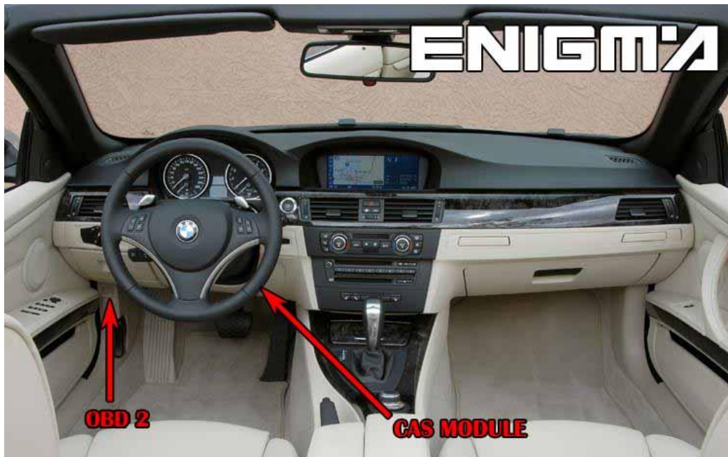
PHOTO 1: Locate the CAS2 module in the car.
