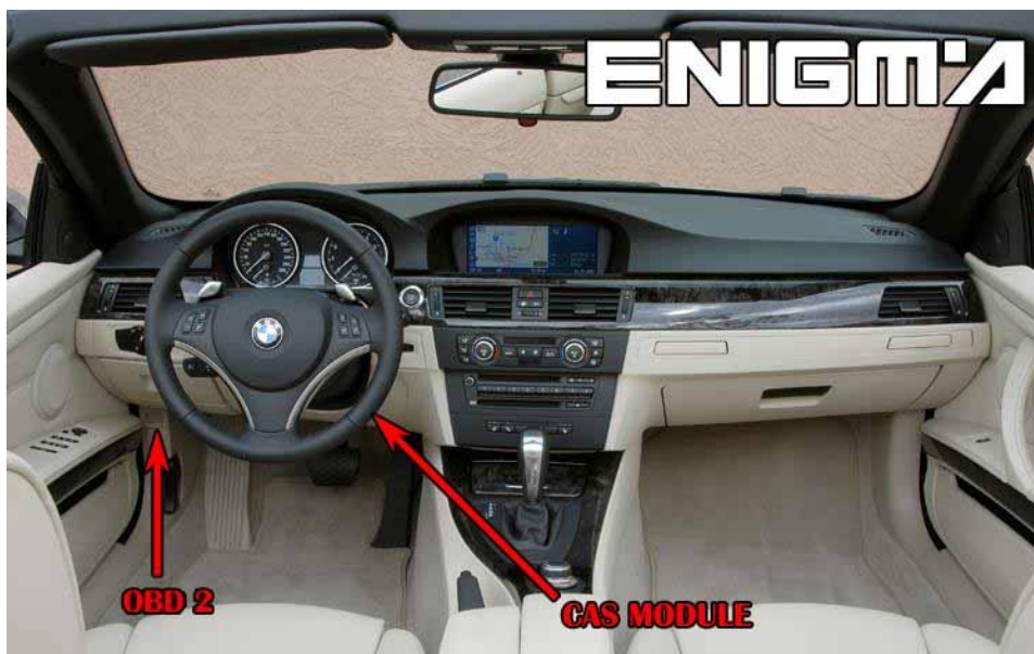
PHOTO 1: Locate the CAS3+ module in the car.
