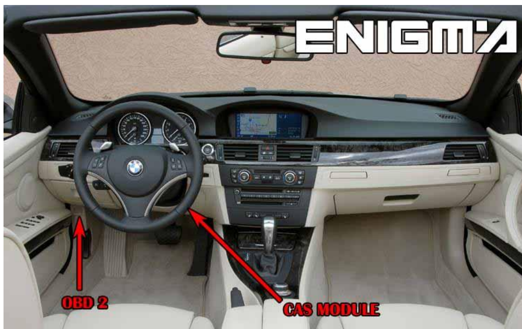
PHOTO 1: Locate the CAS2 module in the car.
