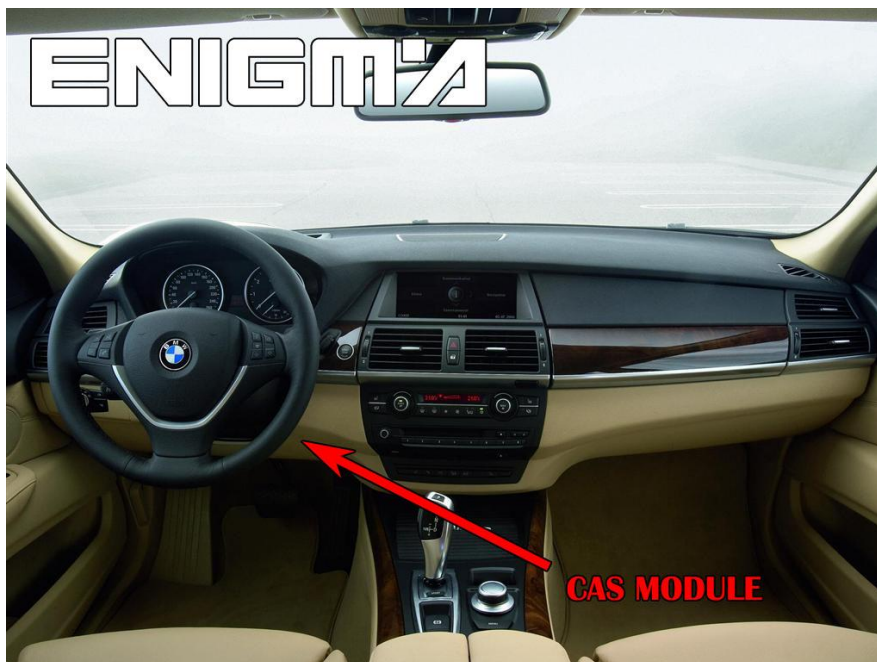
PHOTO 1: Locate the CAS3+ module in the car.
