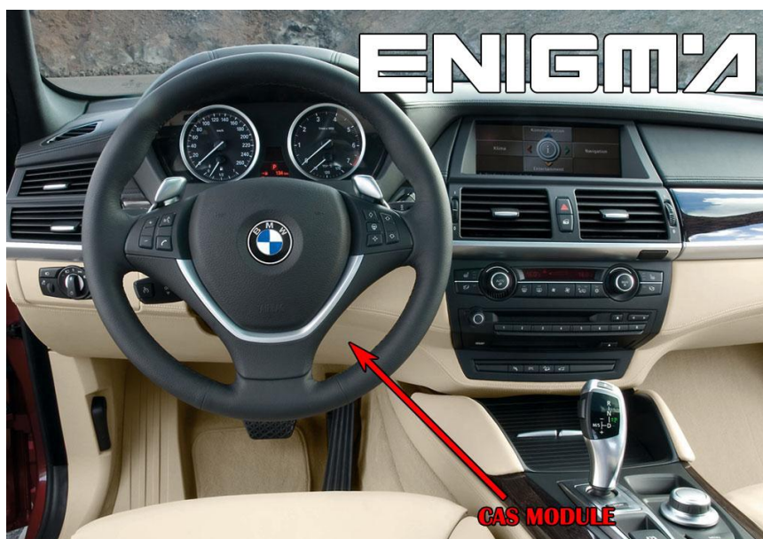
PHOTO 1: Locate the CAS3 module in the car.
