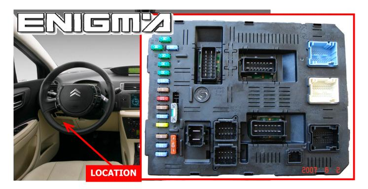
Use cable C4, remove back plastic cover from BSI, then locate eeprom memory and clip it checking pin 1 as shown of photo below:
