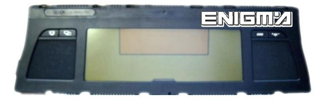
USE CABLE C4, OPEN DASH, PLEASE MAKE IT CAREFULLY, THEN LOCATE EPROM MEMORY 93C66, USUALLY WE DON'T NEED TO DESOLDER IT, AND CLIP IT CHECKING PIN 1 AS SHOWN OF PHOTO BELOW:
