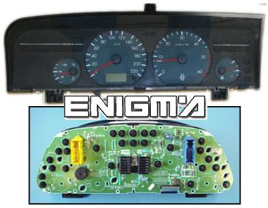
CAREFULLY TAKE OFF BACK FIXED FROM ENGINES, THESE ARE SOME PLASTIC CLIPS THAN JUST NEED TO PRESS, YOU DON'T NEED TO TAKE OFF NAILS, THEN YOU NEED TO TAKE OFF SCREEN CONECTION, AND FINALLY BOARD IS FREE, LOCATE EPROM IN FRONT OF THIS BOARD AND CLIP IT CHECKING PIN 1 AS SHOWN OF BELOW PHOTO:
