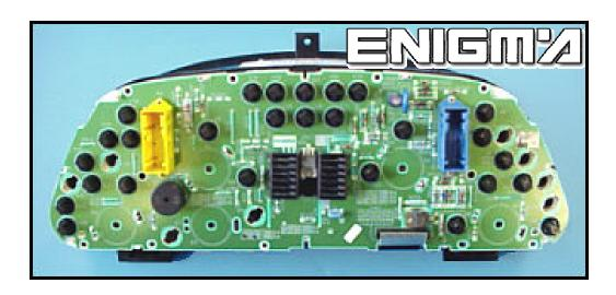
CAREFULLY TAKE OFF BACK FIXED FROM ENGINES, THESE ARE SOME PLASTIC CLIPS THAN JUST NEED TO PRESS, YOU DON'T NEED TO TAKE OFF NAILS, THEN YOU NEED TO TAKE OFF SCREEN CONECTION, AND FINALLY BOARD IS FREE, LOCATE EPROM IN FRONT OF THIS BOARD AND CLIP IT CHECKING PIN 1 AS SHOWN OF BELOW PHOTO:
