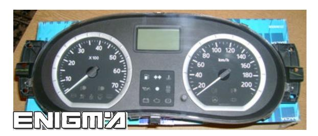
USE CABLE C4, OPEN ALL DASH, PLEASE MAKE IT CAREFULLY, THEN LOCATE EPROM MEMORY 93C56, USUALLY WE DON'T NEED TO DESOLDER IT, AND CLIP IT CHECKING PIN 1 AS SHOWN OF PHOTO BELOW:
