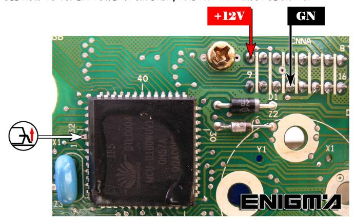
ON NEXT ONE, WE CAN SEE HOW TO SOLDER CABLE LEADS ACCORDING TO COLOURS:
