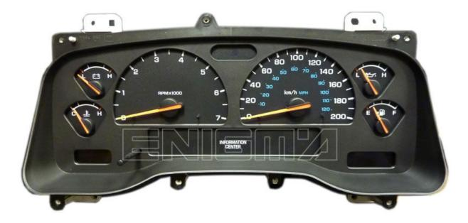
Use cable C5, open back plastic cover from dash, then locate eprom 93C46 memory, and clip it checking Pin 1 as shown of below photo:
