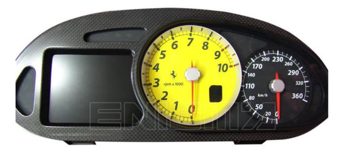
USE CABLE C4, OPEN BACK COVER FROM DASH, CAREFULLY, THEN LOCATE EPROM, AND CLIP IT CHECKING PIN 1 AS SHOWN OF PHOTO BELOW:
