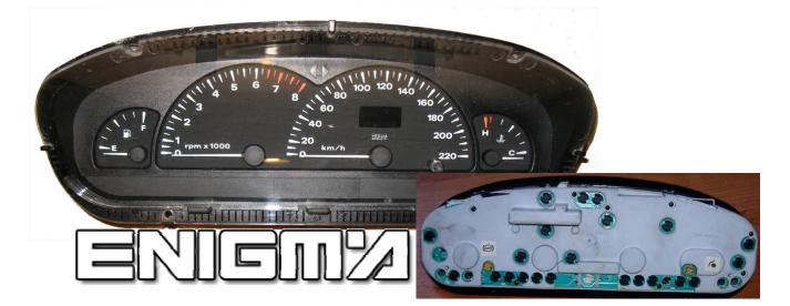
USE CABLE C11, OPEN ALL DASH, PLEASE MAKE IT CAREFULLY, REMOVE CAREFULLY NAILS, ALL THAT WE NEED TILL WE HAVE CLEAN BOARD, AND DISCONNECT SMALL BOARD FROM BIG PART, THEN SOLDER CABLE LEADS ACORDING TO COLOURS AS SHOWN OF PHOTO BELOW IN BOTH SIDES:
