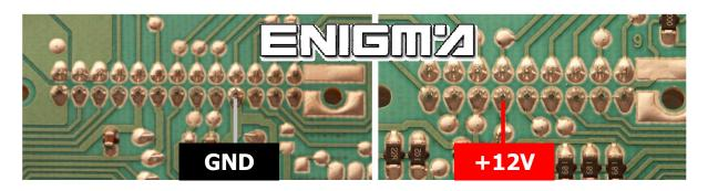
CONNECT OR SOLDER CABLE LEADS ACORDING TO COLOURS AS SHOWN OF PHOTO BELOW, DON'T FORGET TO REALIZE A BRIDGE BETWEEN 2 POINTS:
