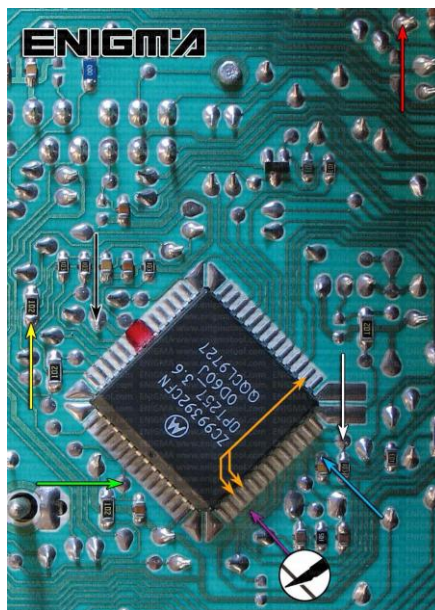
PHOTO 1: Solder cables according to the colors like shown on the photos above.
