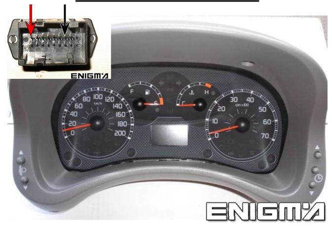
Use cable  ${\it C4}$ , take off dash from car dash, open all dash, please make it carefully. When we have main board on our hands locate eprom memory, and clip it checking pin 1 as shown of photo below:
