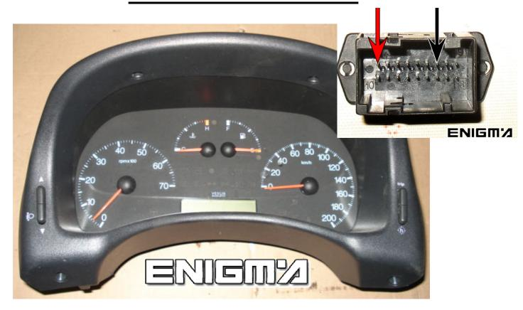
USE CABLE C4, TAKE OFF DASH FROM CAR DASH, OPEN ALL DASH, PLEASE MAKE IT CAREFULLY. WHEN WE HAVE MAIN BOARD ON OUR HANDS LOCATE EPROM MEMORY, AND CLIP IT CHECKING PIN 1 AS SHOWN OF PHOTO BELOW:
