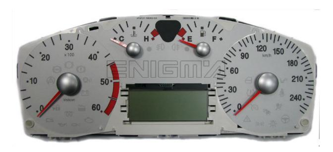
USE CABLE C43, REMOVE OUTSIDE COVERS FROM DASH, THEN CONNECT CABLE PLUG ON PINS ACCORDING TO BELOW PHOTO:
