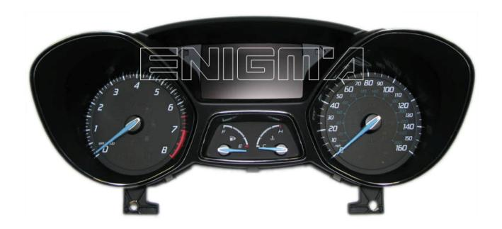
USE CABLE C4, REMOVE ALL PLASTIC COVERS FROM DASH, AND NAILS, CAREFULLY, THEN LOCATE EPROM MEMORY, AND CLIP IT CHECKING PIN 1 AS SHOWN ON BELOW PHOTO:
