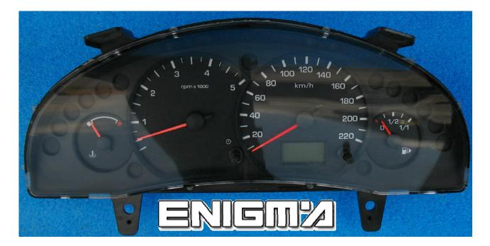
USE CABLE C12, OPEN BACK COVER FROM DASH, THEN CONNECT OR SOLDER CABLE LEADS ACCORDING TO COLOURS AS SHOWN OF BELOW PHOTO:
