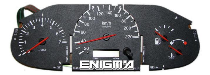
USE CABLE C13 ALWAYS CONNECTED TO A1 ADAPTER. REMOVE BOARD FROM DASH, THEN CONNECT OR SOLDER CABLE LEADS ACCORDING TO NUMBER AS SHOWN IN NEXT PHOTOS:
