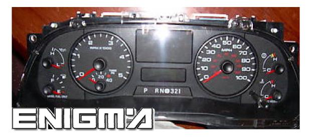
THESE FORD F250 MODELS HAVE SAME OUTSIDE LOOKALIKE DASH AND MICRO INSIDE, BUT BOARDS ARE TWO DIFFERENT VERSIONS. FOR ALL THOSE MODELS WE MUST USE CABLE C12, REMOVE BACK PLASTIC COVER, AND CHECK VERSION LIKE SHOW TO US NEXT INSTRUCTIONS CONNECTING OR SOLDERING CABLE LEADS ACORDING TO COLOURS AS SHOWN ON PHOTOS BELOW:
