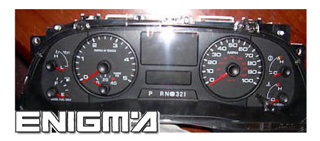
THESE FORD F350 MODELS HAVE SAME OUTSIDE LOOKALIKE DASH AND MICRO INSIDE, BUT BOARDS ARE TWO DIFFERENT VERSIONS. FOR ALL THOSE MODELS WE MUST USE CABLE C12, REMOVE BACK PLASTIC COVER, AND CHECK VERSION LIKE SHOW TO US NEXT INSTRUCTIONS CONNECTING OR SOLDERING CABLE LEADS ACORDING TO COLOURS AS SHOWN ON PHOTOS BELOW:
