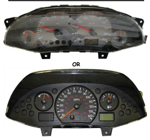
Use specific cable C36, remove dash from car, connect plug into white dash plug, and grey cable to the point show on photo:
