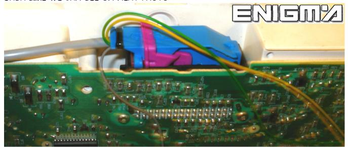
THEN CONNECT OR SOLDER CABLE LEADS ACCORDING TO COLOURS AS SHOWN ON THE PHOTO BELOW:
