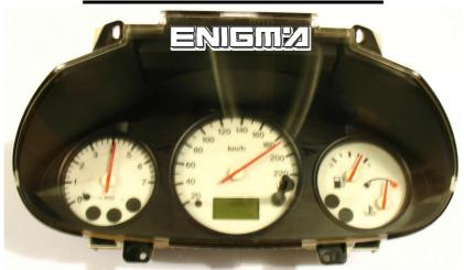
Use specific cable C39, take off from car dash, open back of dash, with 5 torx screws. When back side of board is in front, connect plug to dash like we can see on Next Photo:
