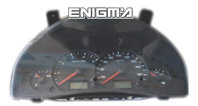
USE CABLE C4, REMOVE DASH FROM CAR, OPEN ALL DASH, PLEASE MAKE IT CAREFULLY. WHEN WE HAVE MAIN BOARD ON OUR HANDS LOCATE EEPROM 24C16 MEMORY, AND CLIP IT CHECKING PIN 1 AS SHOWN OF PHOTO BELOW: AND CLIP IT CHECKING PIN 1 AS SHOWN OF BELOW PHOTO:
