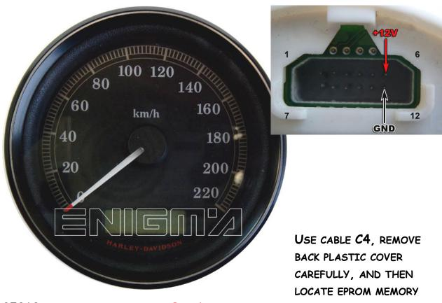
25010, AND CLIP IT CHECKING PIN 1 AS SHOWN OF BELOW PHOTO:
