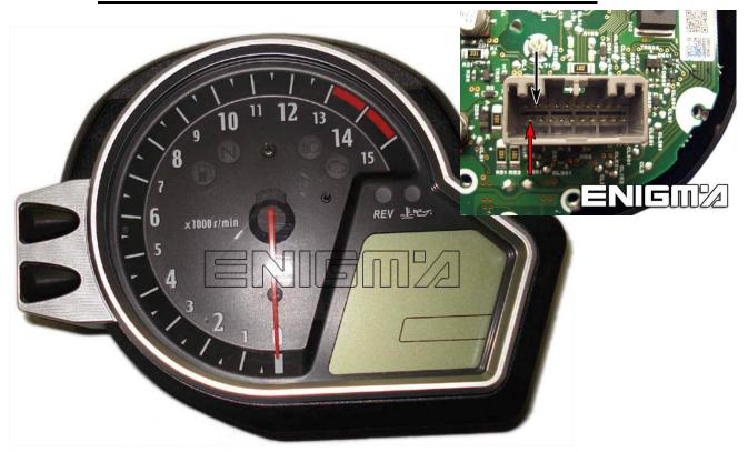
USE CABLE C4, REMOVE BACK COVER, CAREFULLY, THEN LOCATE 93C66 MEMORY EEPROM, AND CLIP IT CHECKING PIN 1 AS SHOWN OF PHOTO BELOW:
