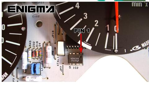
WE CAN ALSO CLIP DIRECTLY, USING CABLE C4, CHECKING PIN 1 POSITION LIKE ON SIDE PHOTO.
