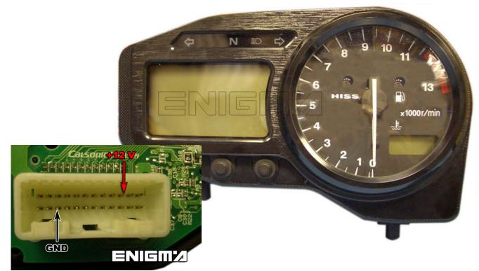
USE CABLE C4, REMOVE BACK COVER, CAREFULLY, THEN LOCATE SL220 MEMORY EEPROM, AND CLIP IT CHECKING PIN 1 AS SHOWN OF PHOTO BELOW:
