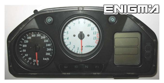
USE **C7** CABLE, REMOVE BACK PLASTIC COVER AND OPEN DASH, THEN LOCATE POINTS AND THEN SOLDER CABLE LEADS ACCORDING TO COLOUR:
