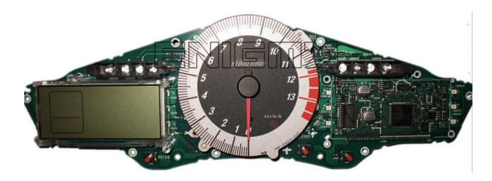
USE C7 CABLE, OPEN BACK COVER OF DASH, LOCATE POINTS IN THE MAIN BOARD LIKE IN PHOTO BELOW AND SOLDER CABLE LEADS AS IT SHOWS TO US:
