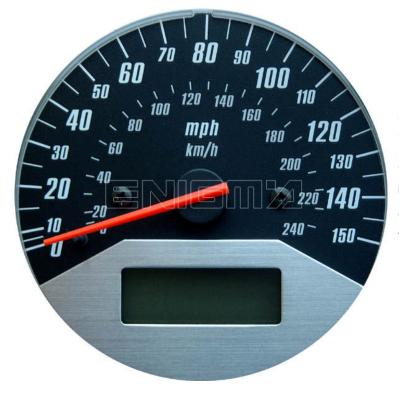
USE CABLE C7, OPEN DASH REMOVING OUTSIDE RING, IT IS VERY DIFICULT, THEN WE CAN SEE THE EPROM MEMORY AND POINTS WHERE WE CAN SOLDER CABLE LEADS ACCORDING TO THEIR COLOURS AS SHOW TO US BELOW PHOTO:
