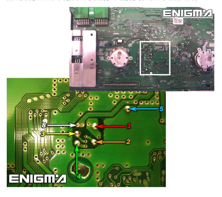
WE CAN USE CABLE C4, OPEN ALL DASH CAREFULLY, THEN LOCATE EEPROM 93C66 OR L56 MEMORY, AND CLIP IT CHECKING PIN 1 AS SHOWN OF BELOW PHOTO:
