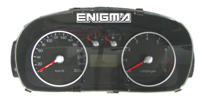
Use cable C5, open back cover from dash, please make it carefully, then locate eeprom 93C46 memory and clip it checking pin 1 as shown of photo below:
