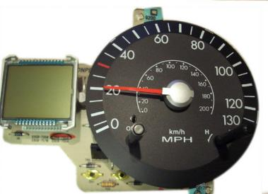
USE C7 CABLE, OPEN DASH AND REMOVE ONLY SPEDOMETER LIKE ON SIDE PHOTO, THEN WE CAN SEE THE 93C46 EPROM, AND WITH THE PHOTO BELOW WE CAN SOLDER CABLE LEADS ACCORDING TO COLOUR:
