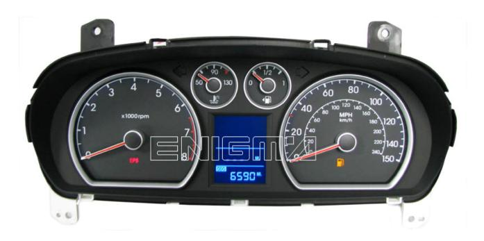
USE CABLE C4, REMOVE BACK COVER FROM DASH, PLEASE MAKE IT CAREFULLY, THEN LOCATE EEPROM 93C56 MEMORY AND CLIP IT CHECKING PIN 1 AS SHOWN ON BELOW PHOTO:
