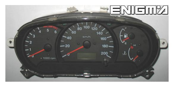
USE CABLE C13 ALWAYS CONNECTED TO A1 ADAPTER. OPEN COMPLETELY DASH, BE CAREFULLY WITH SCREEN, THEN CONNECT OR SOLDER CABLE LEADS ACCORDING TO NUMBER AS SHOWN IN NEXT PHOTO:
