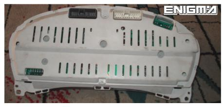
USE CABLE C5, OPEN BACK PLASTIC COVER FROM DASH, BE CAREFULLY, AND THEN LOCATE EPROM 93C46, AND CLIP IT CHECKING PIN 1 AS SHOWN OF BELOW PHOTO:
