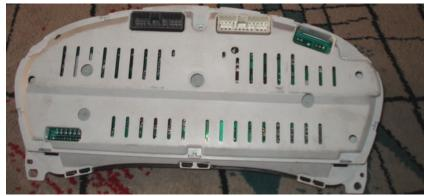
USE CABLE C5, OPEN BACK PLASTIC COVER FROM DASH, BE CAREFULLY, AND THEN LOCATE EPROM 93C56, AND CLIP IT CHECKING PIN 1 AS SHOWN OF BELOW PHOTO:
