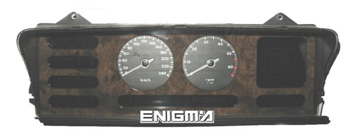
Use cable C5, remove dash from car, this is not so easy, but take some minutes to study, open all dash, please make it carefully, then locate special eprom memory, we don't need to desolder it, and clip it checking pin 1 as shown of photo below:
