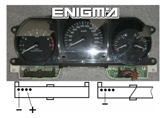
USE CABLE C11, REMOVE BACK COVER FROM DASH, THEN CONNECT OR SOLDER CABLE LEADS ACCORDING TO COLOURS AS SHOWN ON PHOTO, REMEMBER TO LIF UP ONE PIN FROM MICRO:
