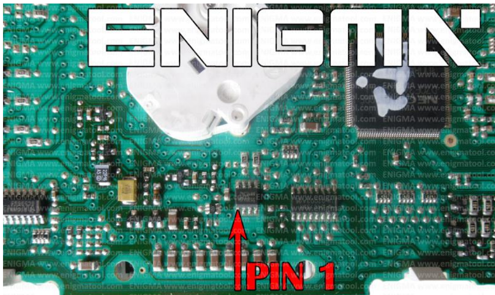
PHOTO 1: Connect cable C4 to the EEPROM memory according to the picture above.
