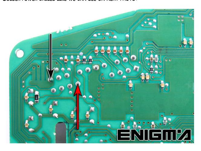
Now we must connect or solder cable leads according to colours as shown on photo below:
