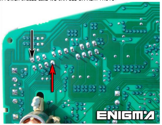
Now we must connect or solder cable leads according to colours as shown on photo below:
